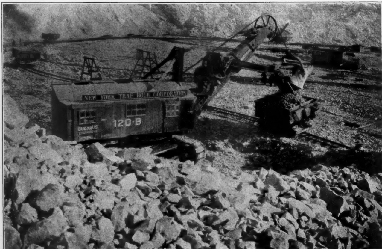
Electric Shovel at Verplank Quarry of the New York Trap Rock Corporation
